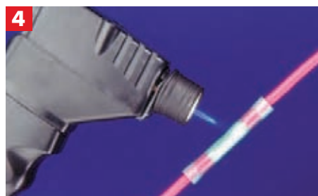
Apply even heat over entire connector.
